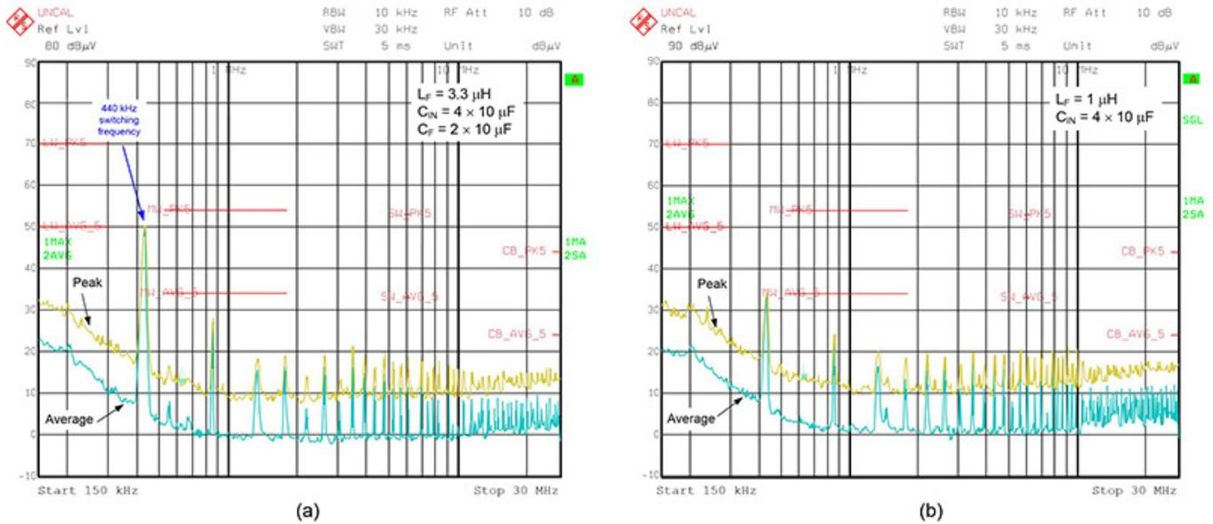
**Figure 2. Comparing a passive filter solution (a) and active filter design (b) using equivalent power-stage operating conditions**
