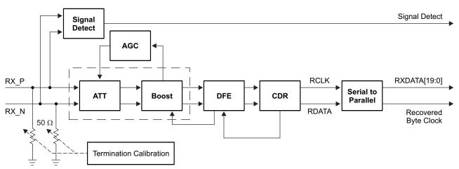
Figure 3. RX Path Block Diagram
