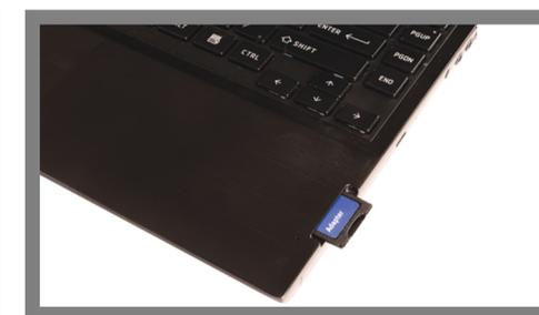
**8** To prepare your workstation for software development, power off the kit, remove the micro SD card; insert it into the included SD card adapter (if applicable); and insert it into your PC. If your PC does not include an SD slot, USB SD card adapters are readily available. Follow the instructions below.
