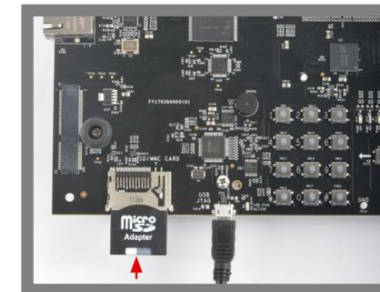
**4** Prepare a Linux µSD card after downloading the software from [www.ti.com/mysecursoftware](http://www.ti.com/mysecursoftware) and following the instructions in the Processor SDK-EPOS Quick Start Guide. Insert the µSD card into the AM438x EVM as shown.
