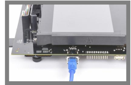
**3** For Linux development, connect the supplied Ethernet cable to the RJ-45 jack on the EVM and the other end to an Internet-enabled router or Ethernet switch. See Section "Linux Software Development Kit."
