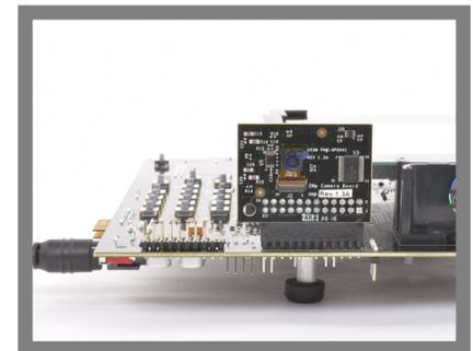
**6** Plug in the camera board (included) as shown. This is only necessary if you plan to run camera application demos.
