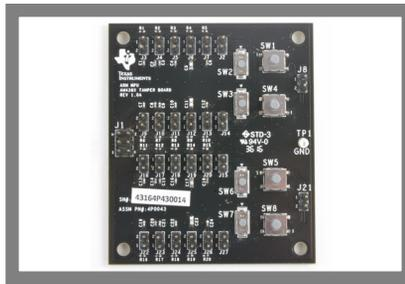
**1** This EVM comes with a coin battery holder. A coin battery is not necessary for normal operation of the EVM. A coin battery (not included) can be inserted for testing ultra-low power (tamper-only) mode.
