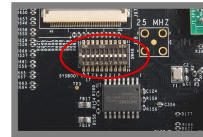
**1** Verify all the SYSBOOT switches are set as shown (all OFF). The switches are on the back of the EVM.
