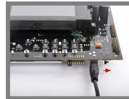
**5** Connect a power supply (not included) to the power jack on the EVM as shown. Turn on the EVM by sliding power switch SW3 to the right position as shown.
