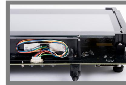
**2** For Linux development, connect the supplied USB cable to the USB connector as shown and the other end to a PC. See Section "Linux Software Development Kit."
