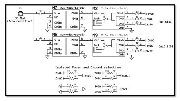
Figure 2-12. Schematic Configuration of Power Supplies
