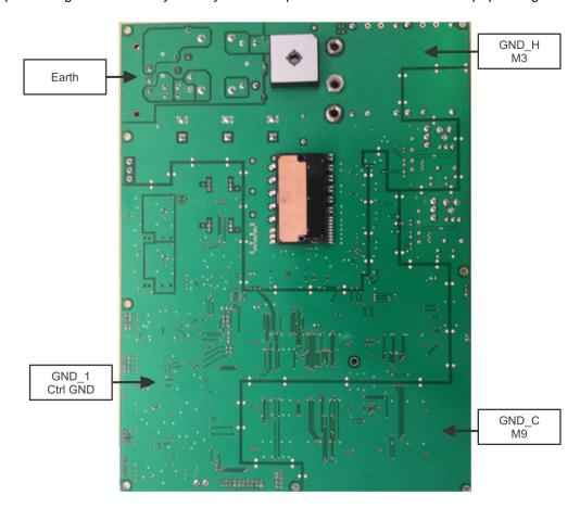
Figure 2-13. Various GND Planes on the Bottom of Board
