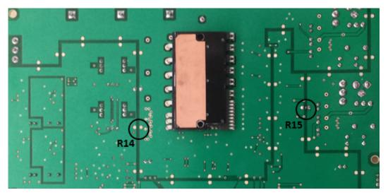
Figure 2-14. Default Connection of Various GND Planes
