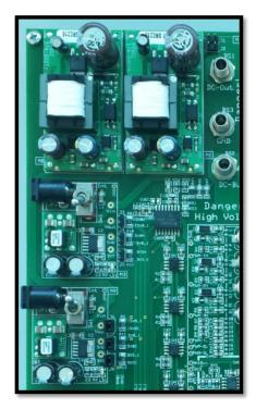
Figure 2-11. Power Supply Block
