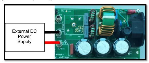
Figure 2-16. Powering Through an External DC Source
