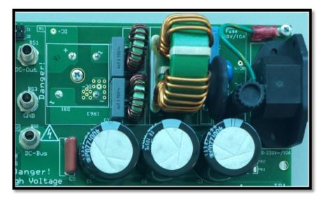
Figure 2-15. AC Line Input Filter and Rectifier
