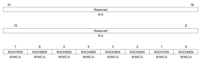
LEGEND: R = Read only; R/W = Read/Write; WC = Write 1 to clear, write of 0 has no effect; -n = value after reset
