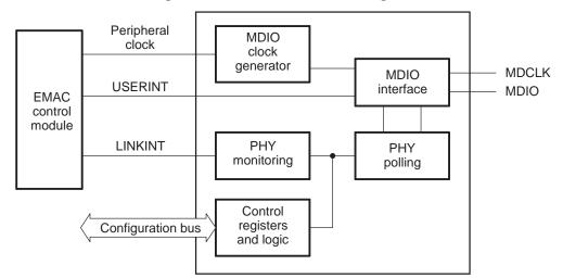
Figure 9. MDIO Module Block Diagram
