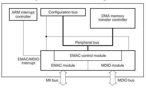
Figure 1. EMAC and MDIO Block Diagram
