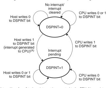
Figure 22. Host-to-CPU Interrupt State Diagram
