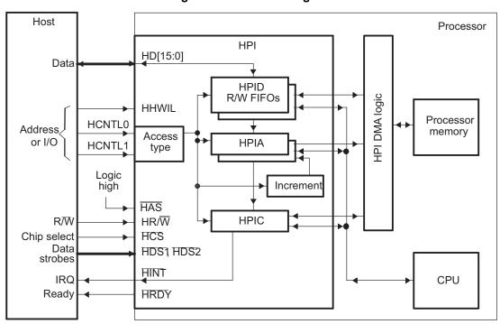
Figure 1. HPI Block Diagram
