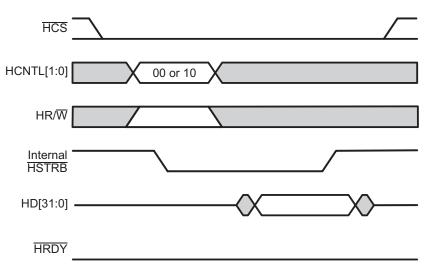
Figure 15 shows an HPIA (HCNTL[1:0] = 10b) write access followed by an HPID (HCNTL[1:0] = 11b) read access for 32-bit multiplexed HPI operation.
