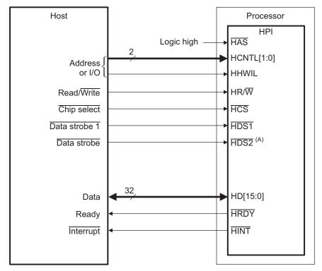
Figure 2. Example of Host-Processor Signal Connections
