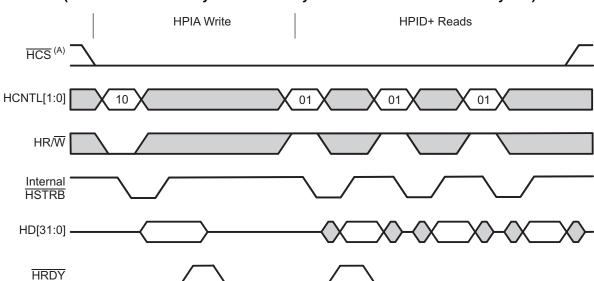
Figure 16. HRDY Behavior During a Data Read Operation in the 32-Bit Multiplexed Mode (Case 2: HPIA Write Cycle Followed by Auto-increment HPID Read Cycles)
