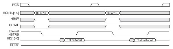
Figure 8 includes an HPID read cycle without auto-incrementing. The host writes the memory address during the HPIA (HCNTL[1:0] = 10b) write cycle, and the host reads the data during the HPID (HCNTL[1:0] = 11b) read cycle. HRDY goes low for each HPIA halfword access, but HRDY goes low for only the first halfword access in each HPID read cycle.
