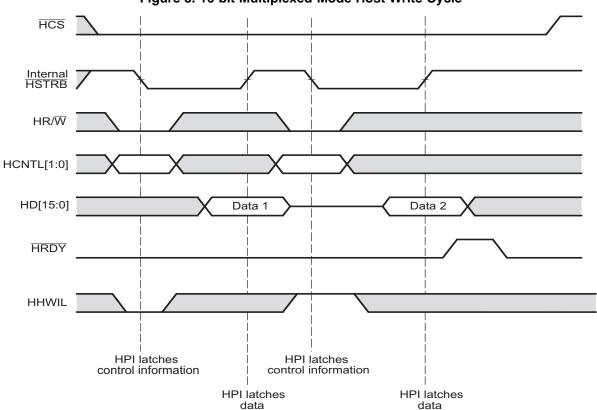
Figure 5. 16-bit Multiplexed-Mode Host Write Cycle
