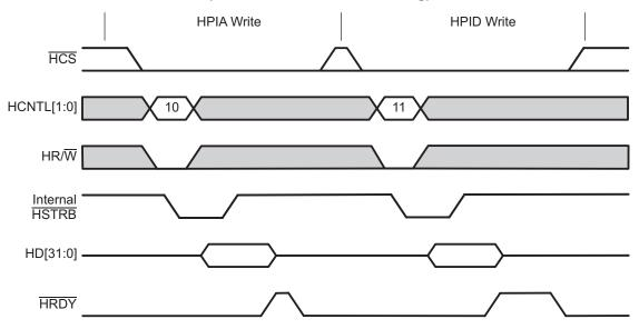
Figure 19 shows an HPIA (HCNTL[1:0] = 10b) write access followed by several auto-incrementing HPID (HCNTL[1:0] = 01b) write accesses when the write FIFO is empty. Note that HRDY is active during the HPIA access but not active during any of the HPID accesses.
