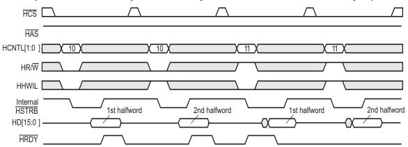
Figure 9 includes an auto-increment HPID read cycle. The host writes the memory address while asserting HCNTL[1:0] = 10b and reads the data while asserting HCNTL[1:0] = 01b. During the first HPID read cycle, HRDY goes low for only the first halfword access, and subsequent HPID read cycles do not cause HRDY to go low.
