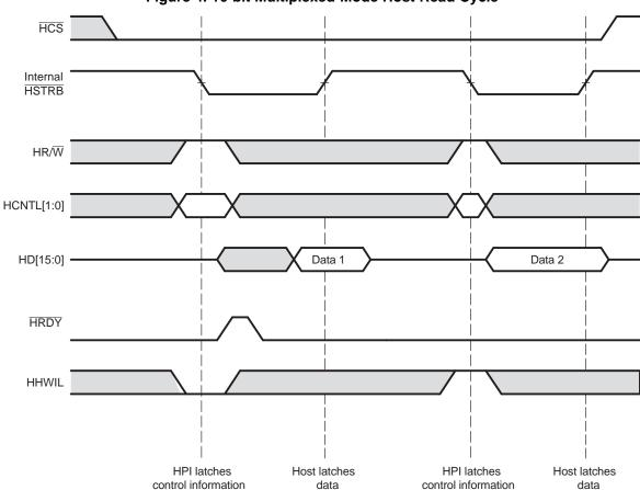
Figure 4. 16-bit Multiplexed-Mode Host Read Cycle
