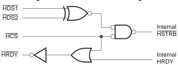
Figure 3. HPI Strobe and Select Logic
