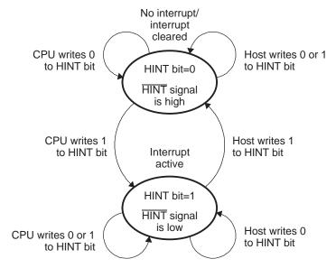
Figure 23. CPU-to-Host Interrupt State Diagram
