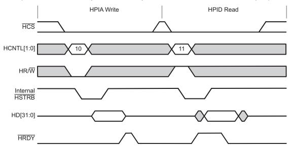
Figure 16 shows an HPIA (HCNTL[1:0] = 10b) write access followed by several auto-increment HPID (HCNTL[1:0] = 01b) read accesses. Note that HRDY is active for the HPIA access. HRDY is also active for the first HPID read access, but not for subsequent read accesses.
