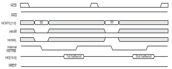
Figure 11 includes a HPID write cycle without auto-incrementing. The host writes the memory address while HCNTL[1:0] = 10b and writes the data while HCNTL[1:0] = 11b. During the HPID write cycle, HRDY goes low only for the second halfword access.
