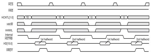
Figure 12 shows auto-increment HPID write cycles when the write FIFO is empty prior to the HPIA write. The host writes the memory address while HCNTL[1:0] = 10b and writes the data while HCNTL[1:0] = 01b. HRDY does not go low during any of the HPID write cycles until the FIFO is full.
