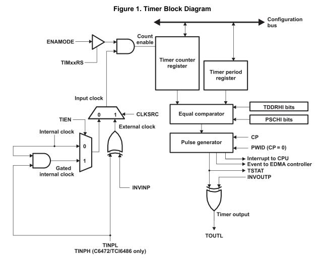
The timer can be driven by an external clock at the timer input pin (TINPL) or by the divide-down clock rate of the internal clock, as shown in Figure 2. For C6472/TCI6486 devices, TINPH can be used to drive the higher 32-bit timer, TIMHI, in unchained mode. The internal clock is generated by the PLL1 controller and is a divided-down version of the CPU clock. For more information, see the device-specific data manual.
