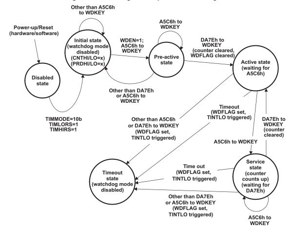
Figure 12. Watchdog Timer Operation State Diagram
