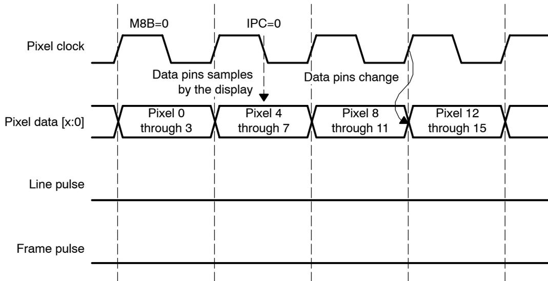
Figure 20. Color Passive Mode Pixel Clock and Data Pin Timing
