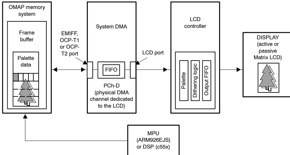
The MPU, or the DSP, stores the image to be displayed in a frame buffer. The frame buffer is used to supply enough encoded pixel values to fill the entire screen at least once.
