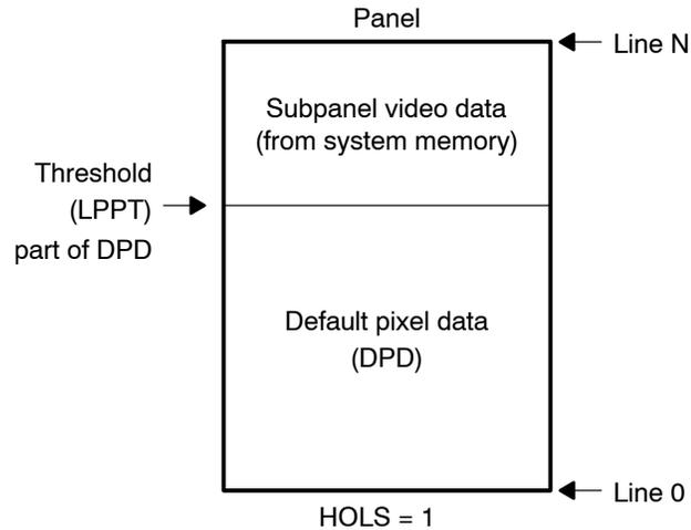
When HOLDS = 0, the beginning of the screen is filled with DPD value until the LPPT excluded. From the LPPT line number, the rest of the screen (below LPPT) displays the image from system memory.
