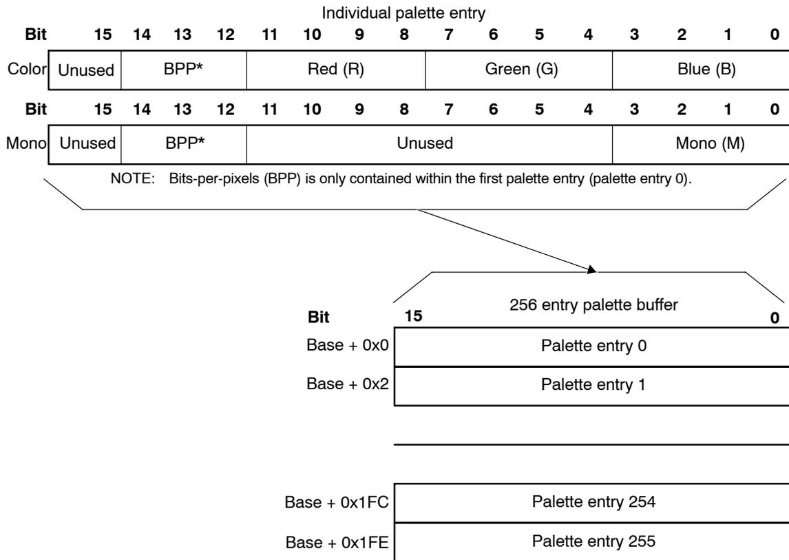
Bits 12, 13, and 14 of the first palette entry select the number of bits-per-pixel to be used in the following frame and thus, the number of palette RAM entries.
