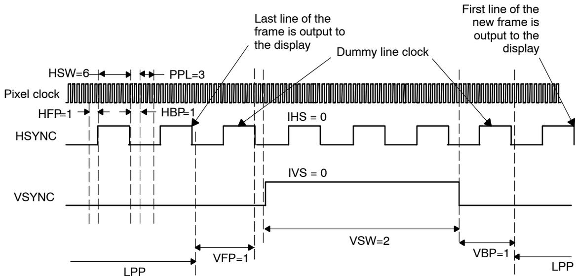
NOTE: Remember that most of the parameters (HSW, HFP, PPL, HBP) must be programmed to value required minus 1.
