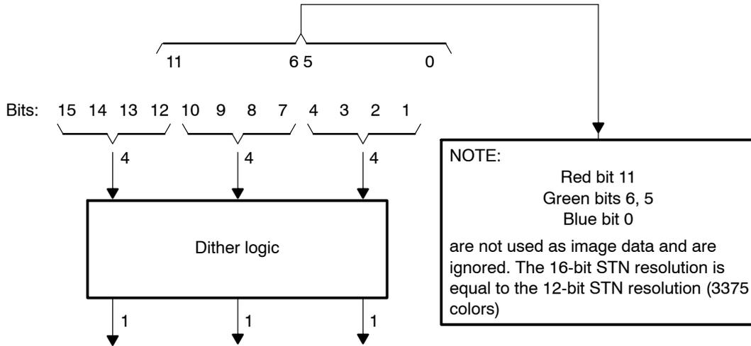
This 12-BPP (5-6-5) mode can be used if the operating system does not support 12 BPP in the frame buffer. Data is arranged in 16 BPP instead, but only 12 bits are dithered and sent to the display.
