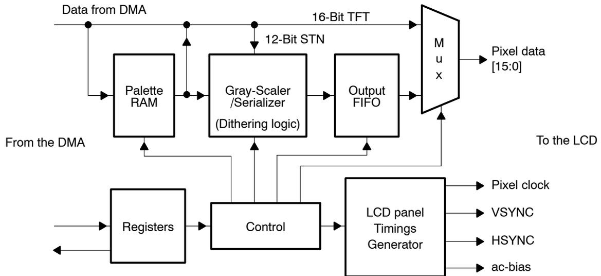
The LCD controller supports single-panel mode displays with programmable sizes. The display can be any width (line length) from 16 to 1024 pixels in 16-pixel increments (bit pixels per line (PPL) in the LCD timing 0 register). The number of lines is set by programming the lines per panel (LPP) field of the LCD timing 1 register (see section 2.3.3, *LCD Timing 1 Register*). The total video frame size is programmable up to 1024 x1024.
