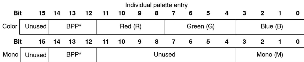
NOTE: Bits-per-pixels (BPP) is only contained within the first palette entry (palette entry 0).
