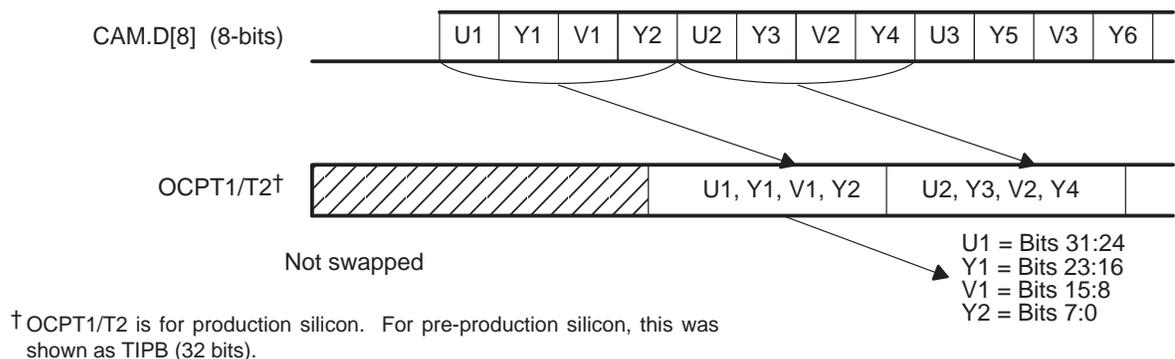
Figure 5. Order of Camera Data on TIPB (Swapped)
