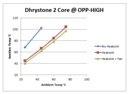
Figure 9. Dyrystone (Core 1 & Core 2) at OPP\_HIGH (Junction Temp vs Ambient Temp)
