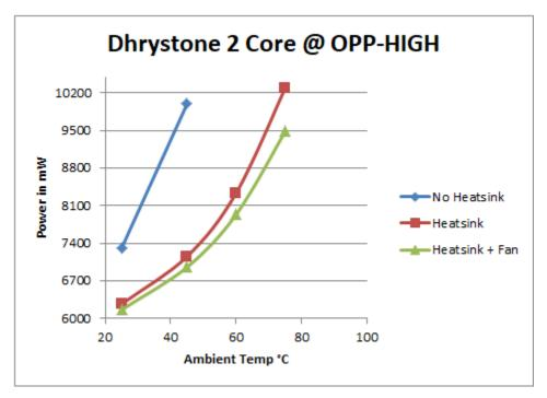
Figure 10. Dyrystone (Core 1 & Core 2) at OPP\_HIGH (Power Consumption vs Ambient Temp)
