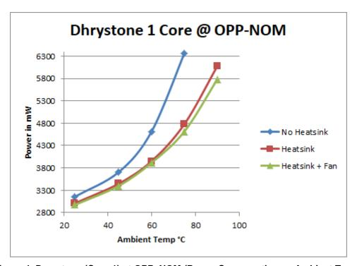
Figure 4. Dyrystone (Core 1) at OPP\_NOM (Power Consumption vs Ambient Temp)
