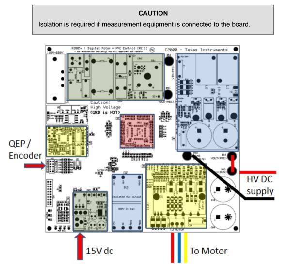
Figure 13. Using External Power Supply to Provide the DC Bus Voltage for the Inverter
