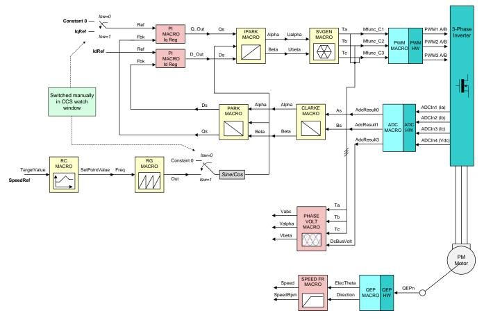
Level 3 verifies the dq-axis current regulation performed by PI macros and speed measurement macros
