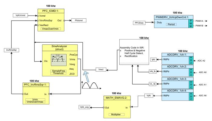
Figure 21. Build 1 Software Blocks
