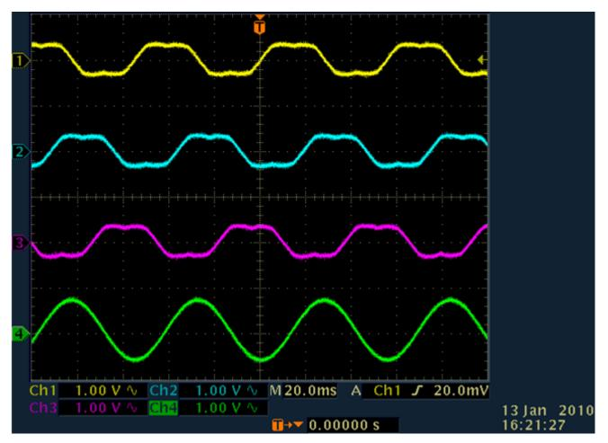
Figure 25. DAC 1 – 4 Outputs Showing Ta, Tb, Tc, and Tb-Tc Waveforms
