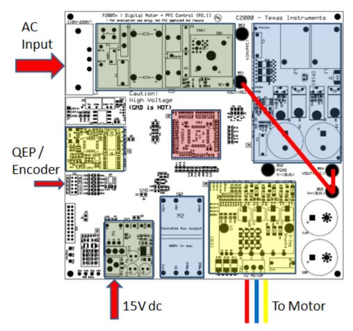
Figure 14. Using AC Input to Generate DC Bus Voltage for the Inverter, Bypassing PFC
