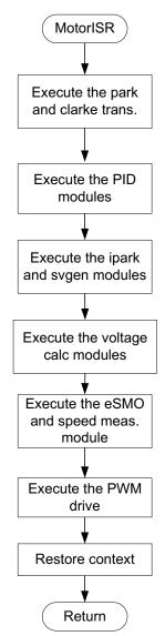
Figure 19. Software Flow for Sensorless PMSM Control
