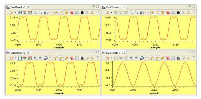
Figure 24. Output of SVGEN, Ta, Tb, Tc, and Tb-Tc Waveforms
