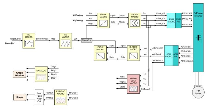
Level 2 verifies the analog-to-digital conversion, offset compensation, Clarke / Park transformations, and phase voltage calculations.
