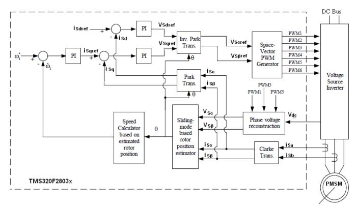
Figure 9. Overall Block Diagram of Sensorless FOC of PMSM
