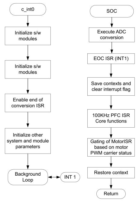
Figure 17. Software Flow Chart for PFC and Motor Control
