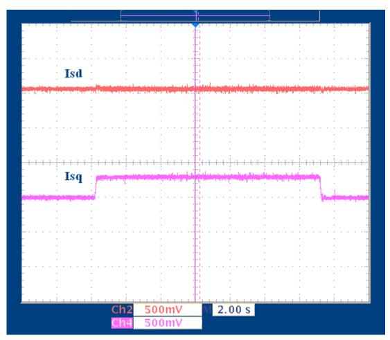
Figure 38. Flux and Torque Components of the Stator Current in the Synchronous Reference Frame Under 0.33-pu Step-Load and 0.5-pu Speed Monitored from PWMDAC Output
