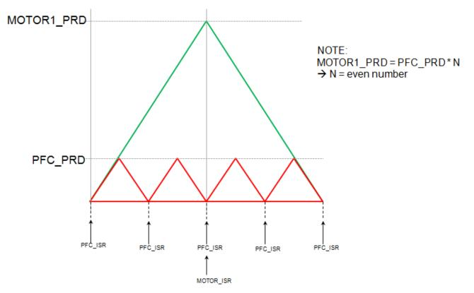
Figure 11. PWM Carrier Alignment for Inverter and PFC
