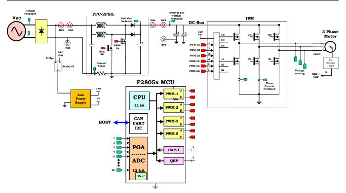
Figure 12. Single-Axis Motor + PFC Board Diagram With F2805x
