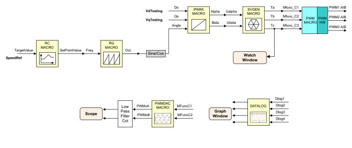
Level 1 verifies the target-independent modules, duty cycles, and PWM updates. The motor is disconnected at this level.
