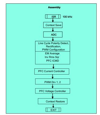
Figure 18. IL PFC Software Flow Diagram
