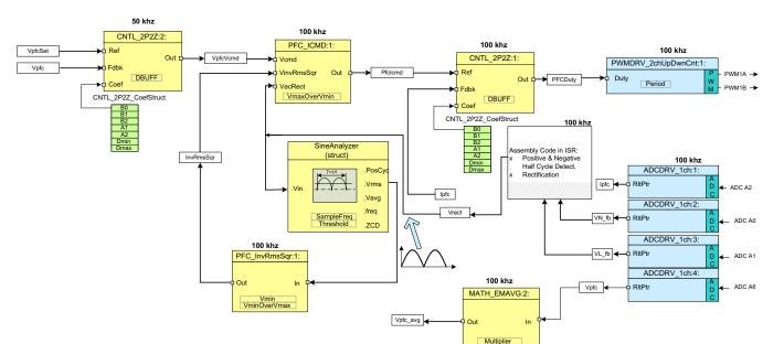
Figure 22. Build 2 Software Blocks
