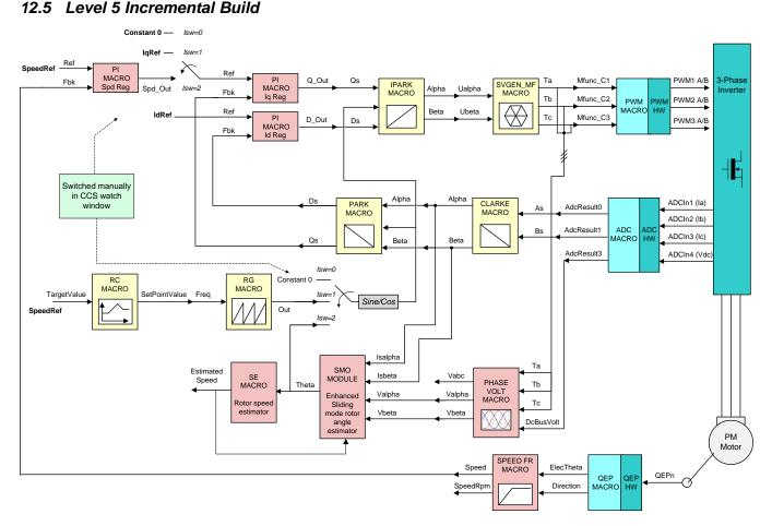
Level 5 verifies the speed PI macro and speed loop. The Speed loop is closed using measured speed as feedback
