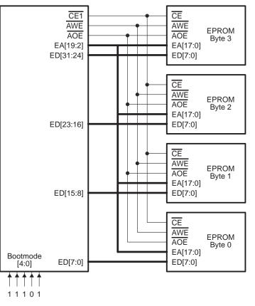
Figure 9. TMS320C6201 Connected to Four 8-Bit EPROM Memories
