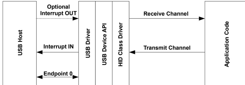
This device class uses one or, optionally, two endpoints in addition to endpoint zero. One interrupt IN endpoint carries HID input reports from the device to the host. Output and Feature reports from the host to the device are typically carried via endpoint zero but devices which expect high host-to-device data rates can select to offer an independent interrupt OUT endpoint to carry these. Endpoint zero carries standard USB requests and also HID-specific descriptor requests.
