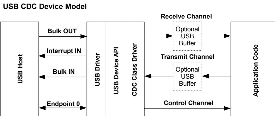
This device class uses three endpoints in addition to endpoint zero. Two bulk endpoints carry data to and from the host and an interrupt IN endpoint is used to signal any serial errors such as break, framing error or parity error detected by the device. Endpoint zero carries standard USB requests and also CDC-specific requests which translate to events passed to the application via the control channel callback.
