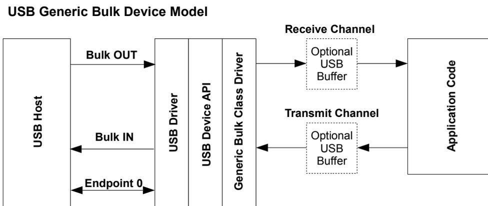
The `usb_dev_bulk` example application makes use of this device class driver.
