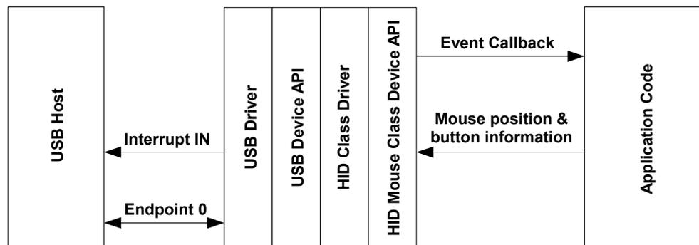
The `usb_dev_mouse` example application makes use of this device class API.
