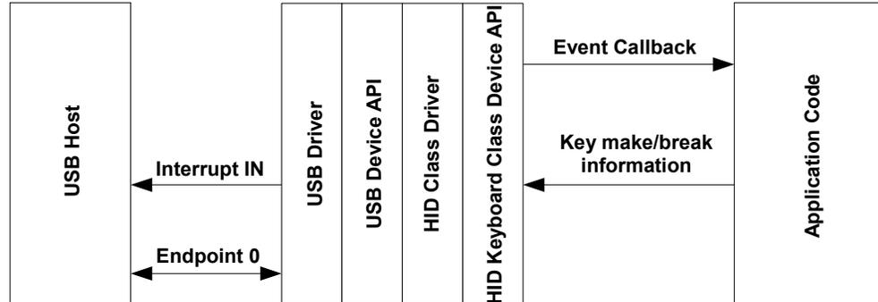
The `usb_dev_keyboard` example application makes use of this device class API.
