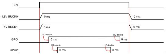
Figure 1. TPS6565342-Q1 Power-up and Power Down Sequence
