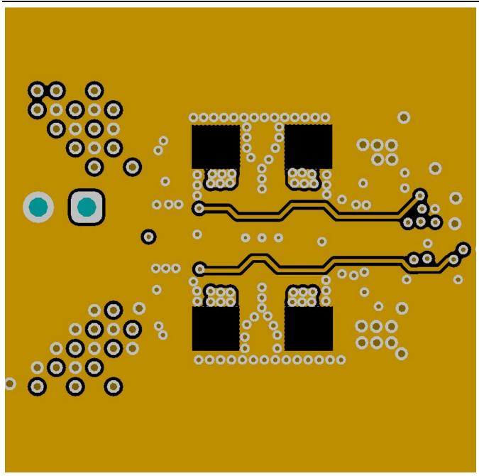
GND plane close to top layer (0.063 mm) helps to reduce parasitic inductance. Holes in the plane are under inductor footprint (SW node) to reduce parasitic capacitance of the SW node, thus reducing noise coupling and improving efficiency.
