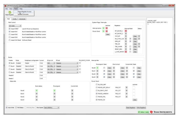
Figure 12. Accessing Direct Register Write
