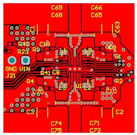
VIN nets are connected to bottom layer with multiple vias. This allows closer placement of the inductors, thus reducing SW node size and EMI. Also snubber circuits are placed next to SW nets for EMI reduction. Multiple GND vias are used to provide solid ground around the LP8756xQ1 device.
