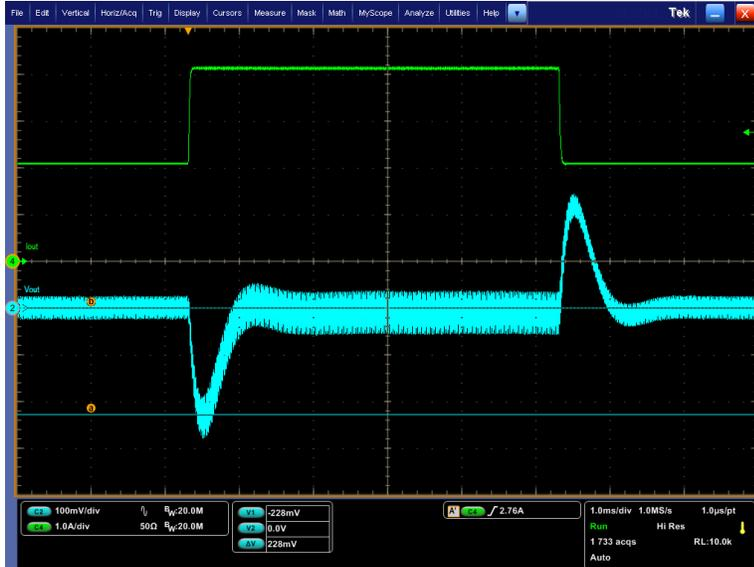
16Vin @ 2A to 4A, 100mA/ $\mu$ s, Pulse f @ 100 Hz,
