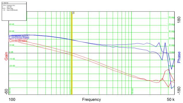
Output power = 24V@0.7AInput voltage = 90VDCPhase margin  $= 64^{\circ}$ Bandwidth = 0.80kHz
