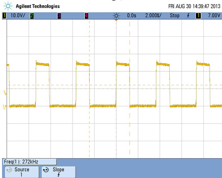
2. Test condition: The input voltage was set at 24V, and all four outputs were set at no load.
