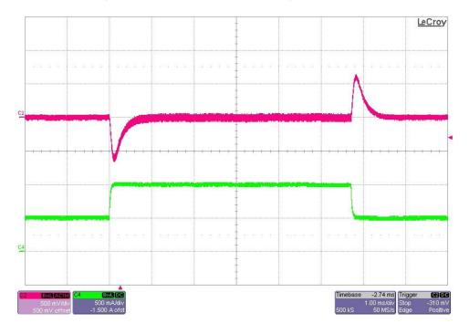
The photo below shows the 12V output voltage (top, ac coupled) when the load current is stepped between 0.5A to 1A. Vin = 24Vdc (500mV/DIV, 500mA/DIV, 1mS/DIV)
