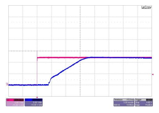
The photo below shows the 12V output voltage startup waveforms after the application of 12Vdc in. The output was loaded with a 1A load. (Vin is 5V/DIV, Vout is 5V/DIV, 5mS/DIV)
