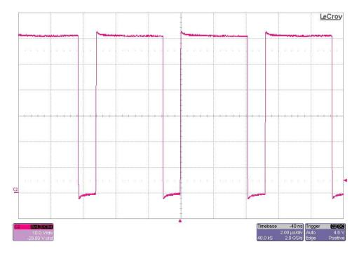
The photo below is the N-ch FET drain waveform. The input voltage is 48V and the output is loaded to 0.45A (the converter is entering discontinuous operation). (10V/DIV, 2uS/DIV)
