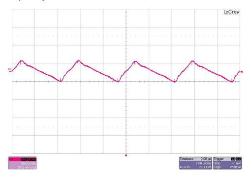
The 12V output ripple voltage is shown in the figure below. The image was taken with the output loaded to 1A and the input voltage set to 12Vdc. (100mV/DIV, 2uS/DIV)
