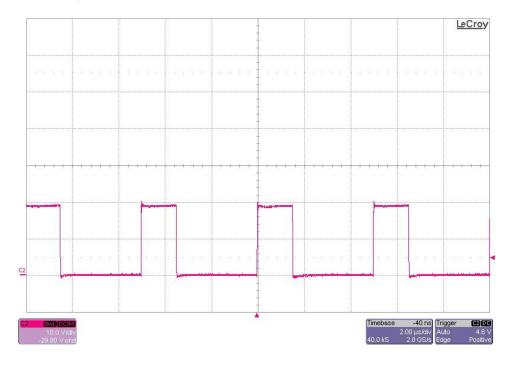
The photo below is the N-ch FET drain waveform. The input voltage is 6V and the output is loaded to 0.067A (the converter is entering discontinuous operation). (10V/DIV, 2uS/DIV)
