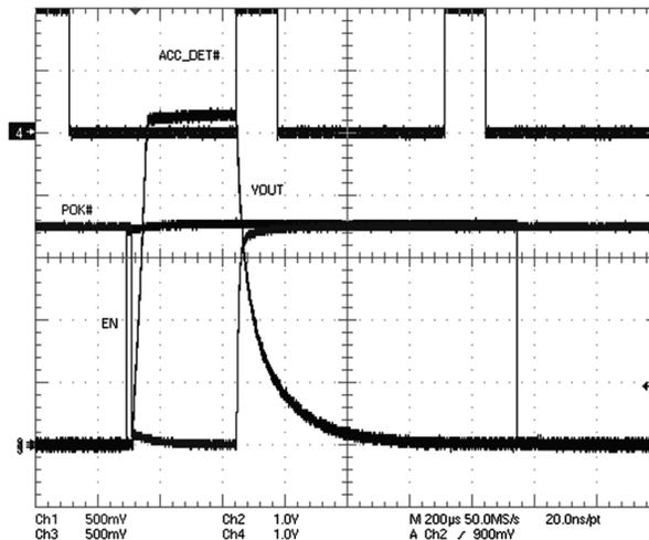
Figure 9. ENABLE and ACC\_DET Cycled Independently, VCC = 5.3V
