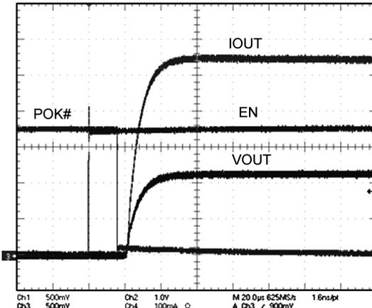
Figure 7. ENABLE Turn On Into An Overload Condition (4Ω Resistive Load), VCC = 5.3V
