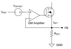
Figure 3. Offset Voltage Model
