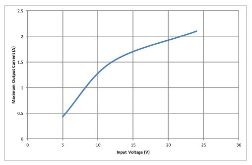
Figure 6. Maximum Output Current Vs. Input Voltage
