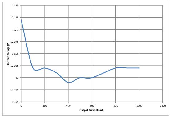
Figure 5 shows the load regulation of the design with the input voltage set to -12V.
