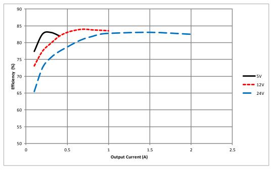
Figure 4. Efficiency Vs. I<sub>OUT</sub>, V<sub>OUT</sub> = -12V
