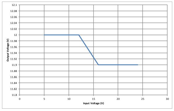
Figure 3. Line Regulation, I<sub>OUT</sub> = 400mA
