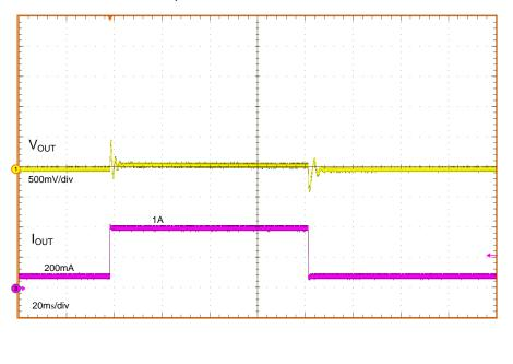
Figure 7. Load Transient  $V_{IN}$  = -12V,  $V_{OUT}$  = -12V,  $I_{OUT}$  = 200mA to 1A
