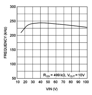
Figure 4. Frequency vs Input Voltage
