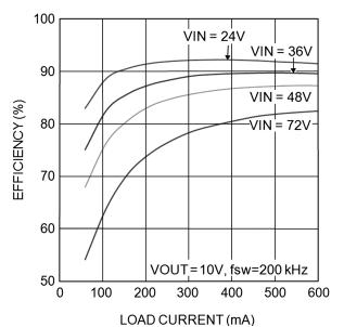
Figure 3. Efficiency vs Load Current
