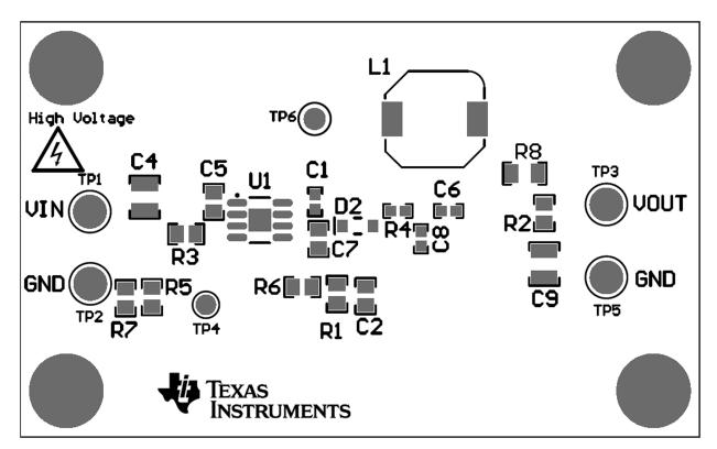
Figure 1. Evaluation Board (Top View)
