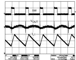
Figure 5. Typical Switching Waveform ( $V_{IN} = 48 \text{ V}, I_{out} = 200 \text{ mA}$ )
