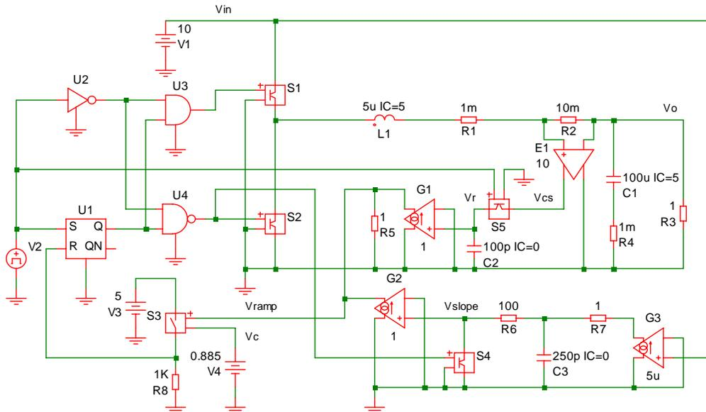
Figure 6: SIMPLIS SPICE schematic - emulated peak current mode synchronous buck.
