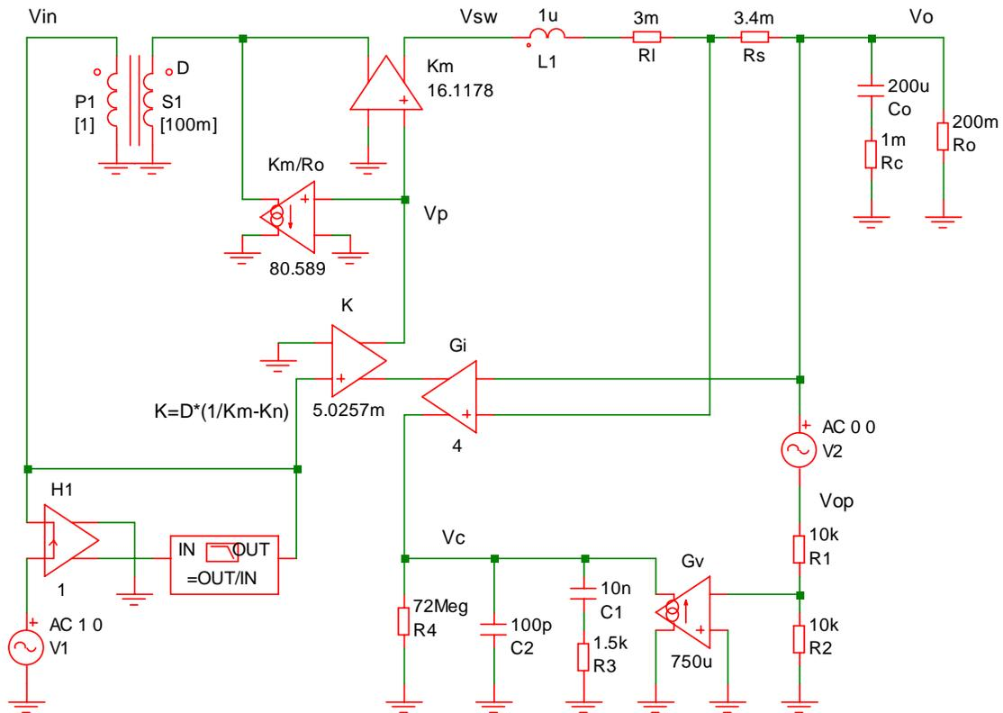
Figure B-9: SIMETRIX LM3495 Linear Model for Input Impedance
