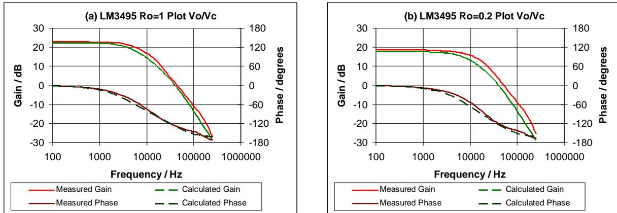
Figure 15: LM3495 control to output gain.
