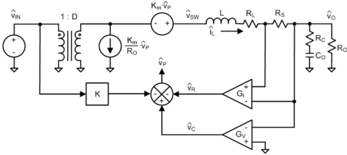
Figure A-4: Complete low frequency unified buck regulator linear model using general gain parameters. To model the current loop with sampling gain term, multiply  $K_m$  by  $H_p(s)$  (valid for PCM1, VCM1 and VCM3 only). To model the control to output or voltage loop with sampling gain term, multiply  $G_i$  by  $H(s)$ .
