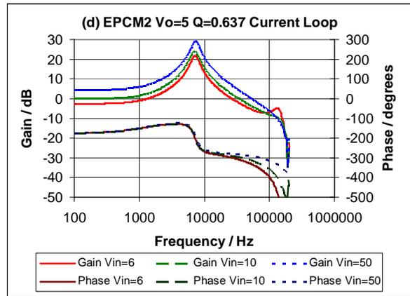
Figure 9: SIMPLIS SPICE results of current loop gain.
