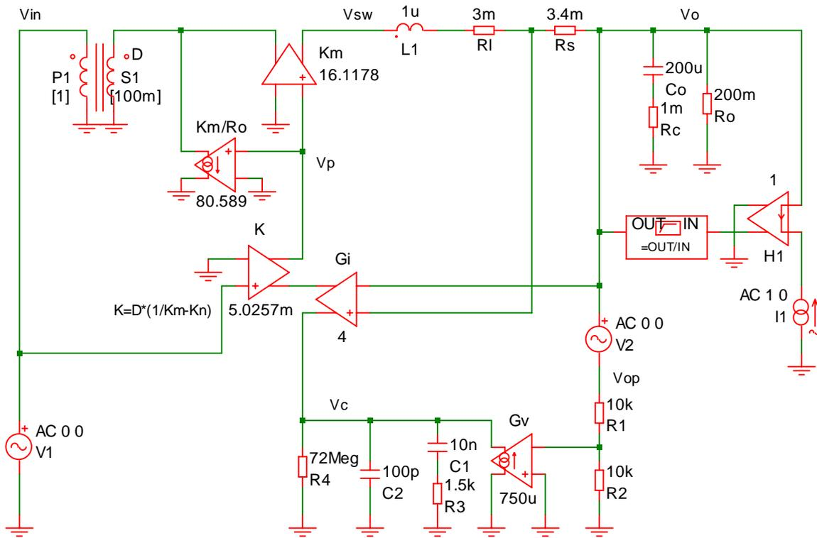
Figure B-7: SIMNETRIX LM3495 Linear Model for Output Impedance
