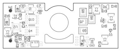
Figure 13. Bottom Layer Assembly
