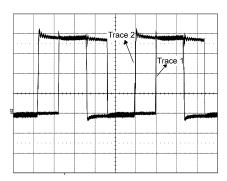
Conditions: Input Voltage=75V Output Current=10A Trace 1: SW1 Node Q2 Drain Voltage Volts/div=20V Trace 2: SW2 Node Q3 Drain Voltage Volts/div=20V Horizontal Resolution=1 µs/div
