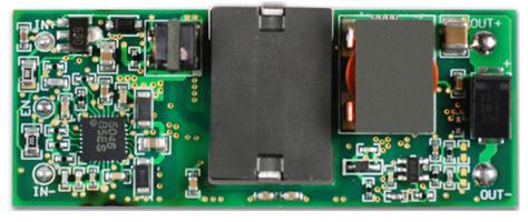
Figure 2. LM5046 Based Eighth Brick Reference Board
