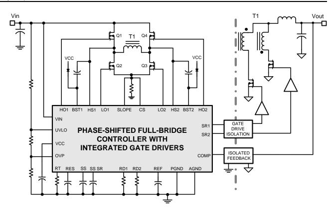
Figure 1. Simplified Phase-Shifted Full-Bridge Converter
