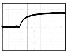
Conditions: Input Voltage=48V Output Current=12A Trace 1: Output Voltage Volts/div=5V Horizontal Resolution =1.0 ms/div
