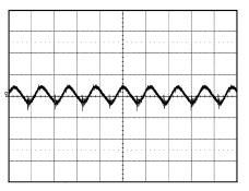
Conditions: Input Voltage=48V Output Current=12A Bandwidth Limit=20 MHz Trace 1: Output Voltage 100 mV/div Horizontal Resolution=2 µs/div
