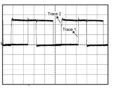
Conditions: Input Voltage=48V Output Current=10A Trace 1: SW1 Node Q2 Drain Voltage Volts/div=20V Trace 2: SW2 Node Q3 Drain Voltage Volts/div=20V Horizontal Resolution=1 µs/div
