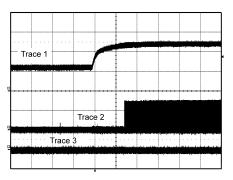
Conditions: Input Voltage=48V, Output Pre-Bias=6V Trace 1 (Channel 1): Output Voltage Volts/div=5V Trace 2 (Channel 2): SR gate Volage Volts/Div=5V Trace 3 (Channel 3): Output Current Amps/div=200mA Horizontal Resolution=2.0 ms/div
