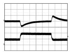
Conditions: Input Voltage=48V Output Current=5A to 10A to 5A Upper Trace: Output Voltage Volts/div=500mV Horizontal Resolution=200 µs/div
