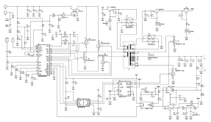
Figure 11. LM5046 Based Eight Brick Reference Board Schematic
