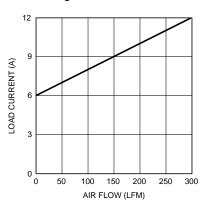
Figure 10. Load Current vs. Air Flow
