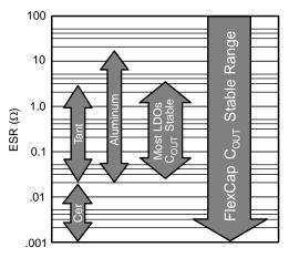
Figure 1. ESR Ranges for Various Output Capacitor Types
