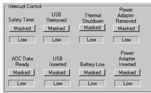
Figure 9. Interrupt Control Interface
