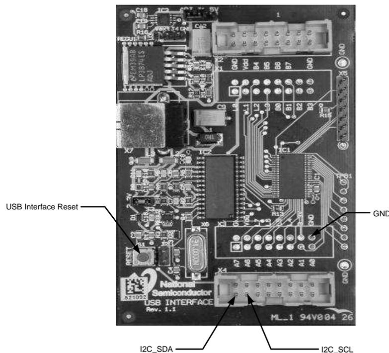
**Figure 2. USB Interface Board**
