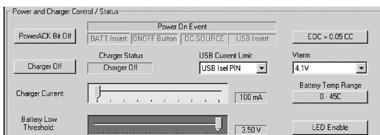
**Figure 7. Battery GUI Interface**
