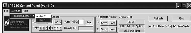
Figure 11. USB Regulator voltage select
