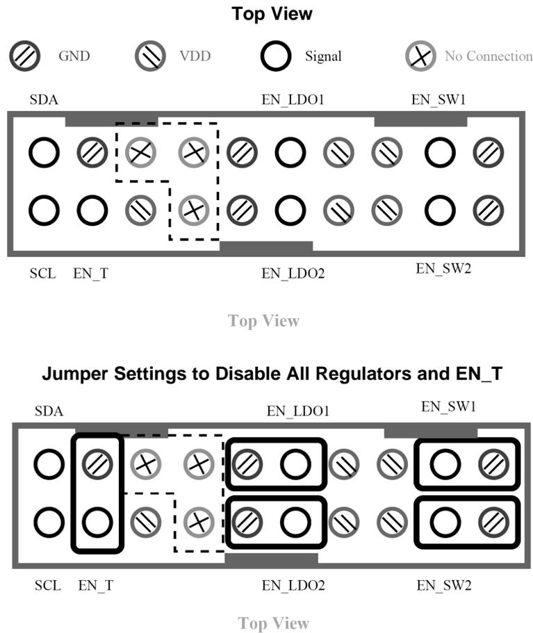
**Figure 10. Header Connector**
