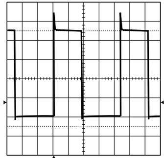
**Figure 6. Drain Voltage**
