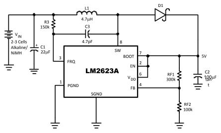
Figure 1. LM2623 Boost Converter for Digital Camera Motor
