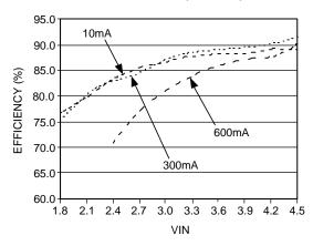
Figure 2. Efficiency for LM2623A Ratio Adaptive Circuit
