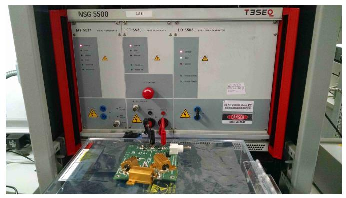
Figure 1. TLV1805-Q1 EVM Setup on Teseq NSG5500 Test System
