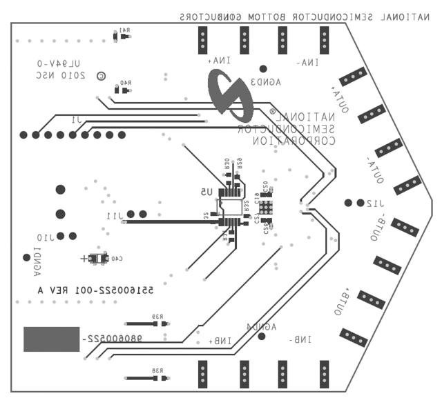
Figure 5. Evaluation Board Bottom Layer
