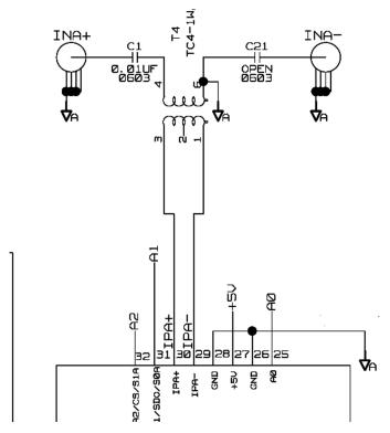
Figure 3. Input Schematic
