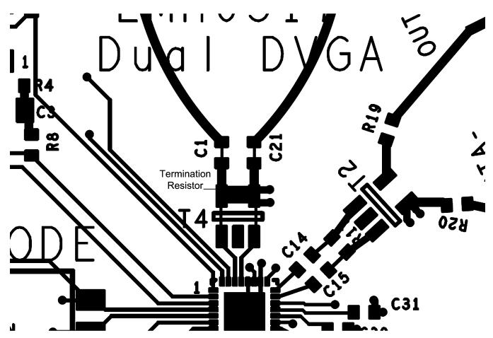
**Figure 6. Connections for Differential Input**
