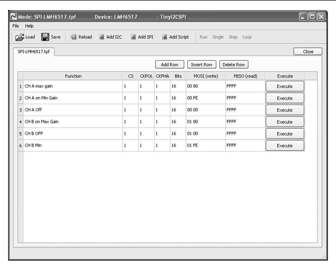
Figure 9. Software Settings for SPI Control
