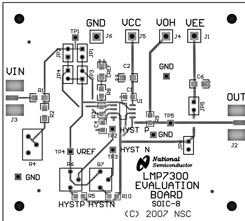
Figure 3. SOIC Top Layer
