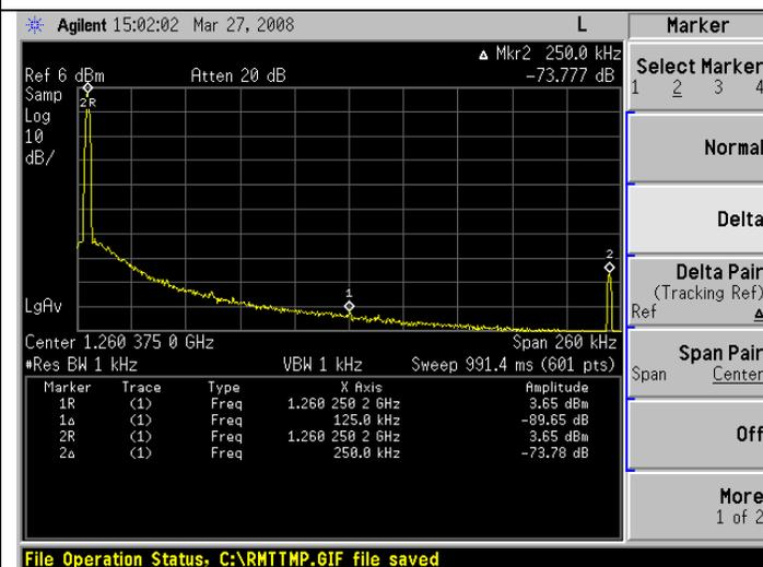
Fractional Spur at 250 kHz offset at a worst case frequency of 1260.25 MHz is  $-73.8$  dBc.
