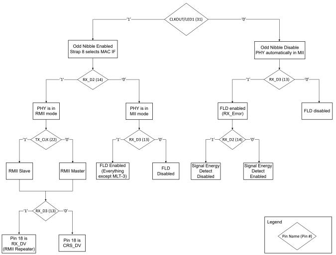
Figure 3-6. DP83826 Enhanced Mode Strapping Flowchart
