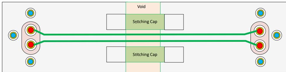
**Figure 19-3. Stitching Capacitor over Plane Split**
