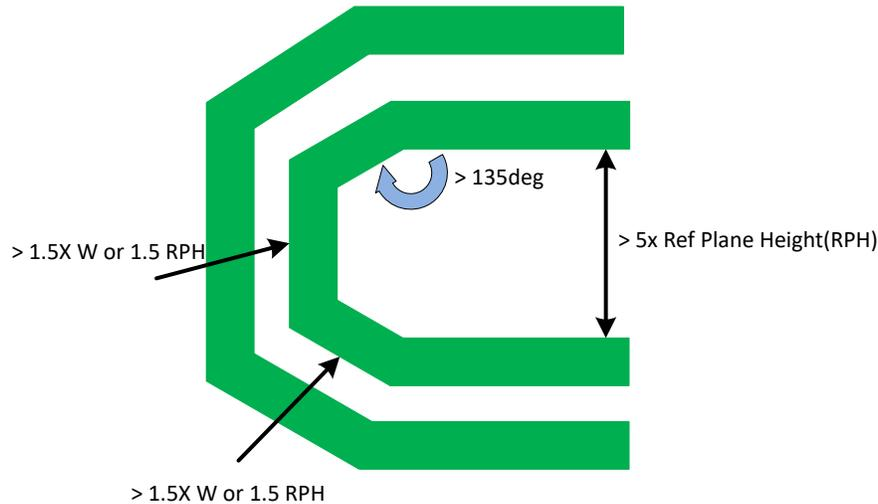
**Figure 16-1. Shortest Trace Length Example**
