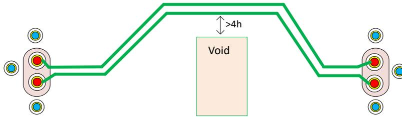
**Figure 19-2. Correct Plane Voiding**
