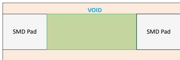
**Figure 26-1. Reference Plane Void Example**
