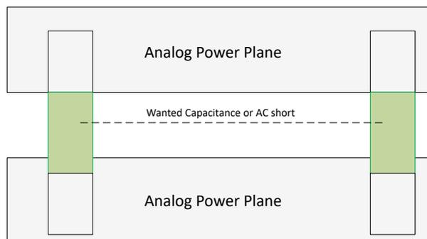
**Figure 19-4. Passed Capacitance Examples**
