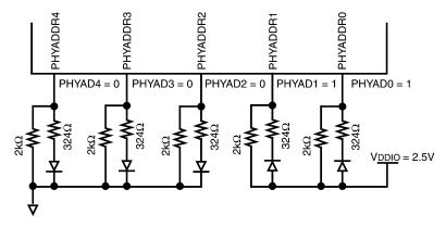
Figure 10. PHYAD/LED Strap Configuration. (PHY base address = 3)
