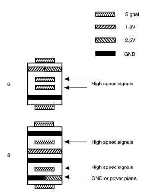
Figure 5. PCB Layer Stacking, Circuit Side
