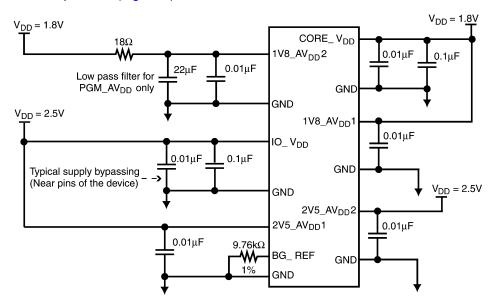
Figure 3. Power Supply Filtering (One Port)
