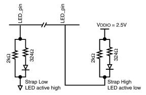
Figure 11. LED/Strapping Option examples
