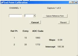
Figure 4-7: Calibration Window with previous Data Points in Display.
