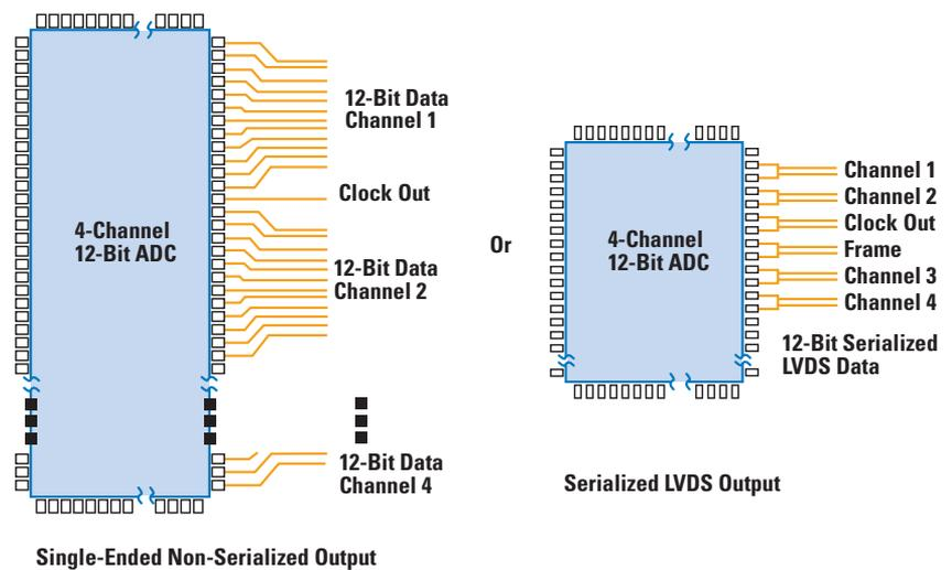
Figure 3. CMOS vs LVDS Board Layout Comparison
