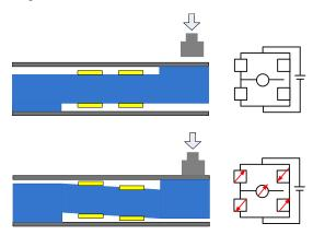
Figure 1. Load Cell Mechanism
