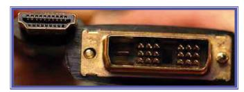
Digital Visual Interface (DVI) has been popular in the computing segment for a number of years. The interface consists mainly of three differential data lines and one differential clock. Each data line has a data rate of up to 1.65Gbps, while the differential clock can run up to 165MHz. This gives an overall throughput of 4.95 Gbps, which is ideal for digital video.
