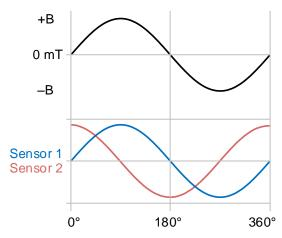
Figure 7. Output from Two Linear Hall Sensors
