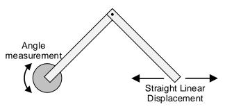
Figure 4. Linear Displacement in a Straight Line
