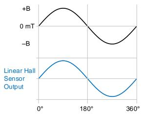
Figure 6. Output from One Linear Hall Sensor
