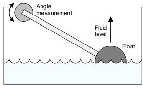
Figure 3. Fluid Level Described By Angle
