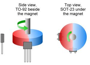
Figure 8. Sensor Placement Examples
