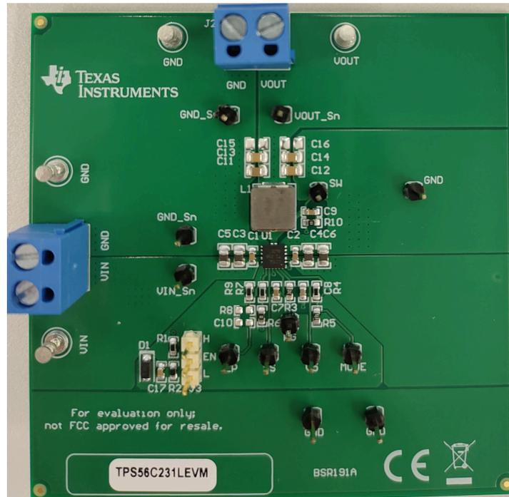
**Figure 6-1. Top View of TPS56C231LEVM**
