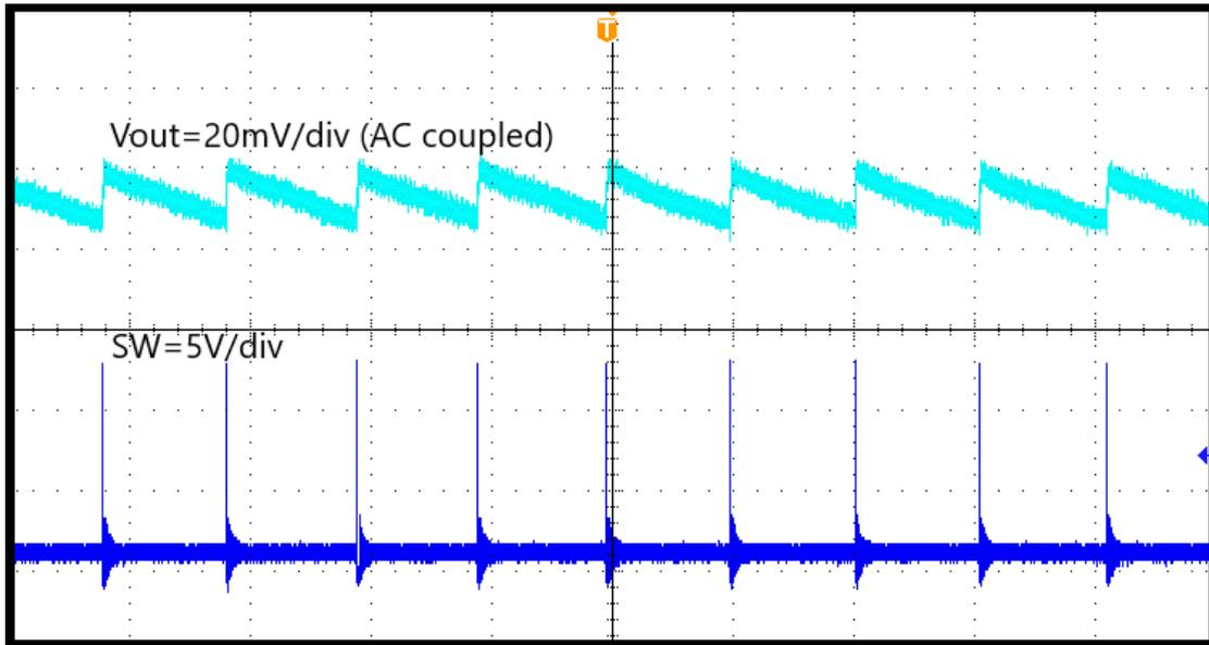
Figure 4-3. TPS56C231L Output Voltage Ripple,  $I_{OUT} = 0.01\text{ A}$  (80  $\mu\text{s}/\text{div}$ )
