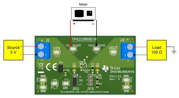
Figure 6-1. Ron Test Setup
