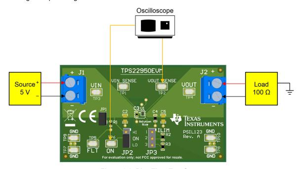
Figure 6-2. Rise Time Test Setup
