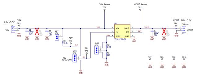
Figure 3-1. TPS22950Q1EVM Schematic
