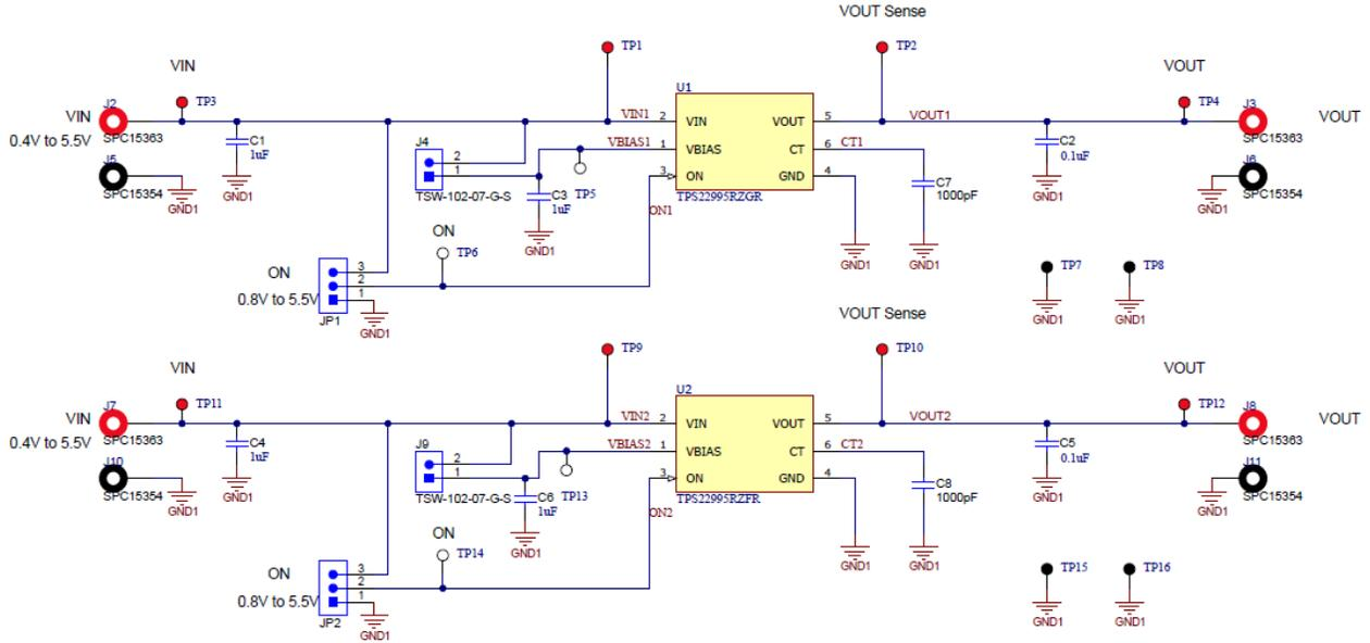
Figure 3-1. TPS22995EVM Schematic
