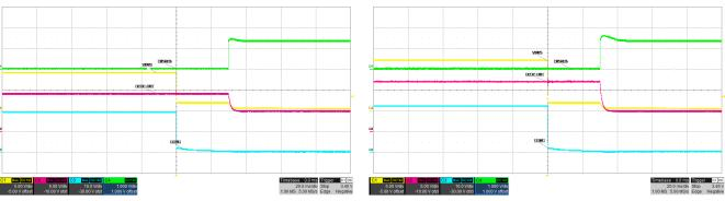
Figure 26. 5-A Transient Triggers OCP at 9 V
