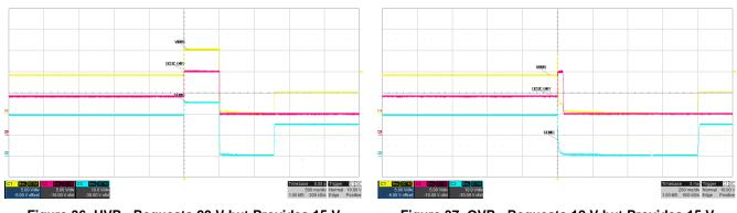
Figure 36. UVP - Requests 20 V but Provides 15 V
