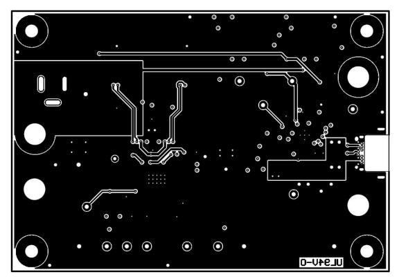
Figure 43. Bottom Side Routing
