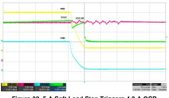
Figure 32. 5-A Soft Load Step Triggers 4.2-A OCP at 20 V
