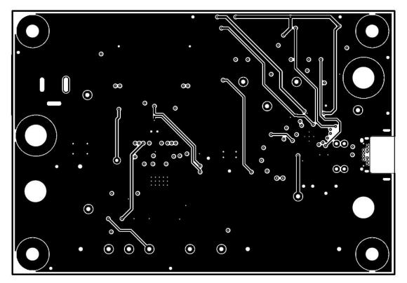
Figure 42. Layer Three Routing
