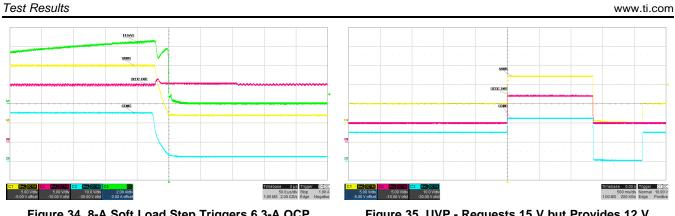
Figure 34. 8-A Soft Load Step Triggers 6.3-A OCP at 15 V
