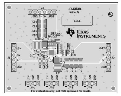
Figure 4. Top Assembly Layer
