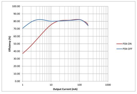
Figure 3. TPS65131 VNEG Efficiency
