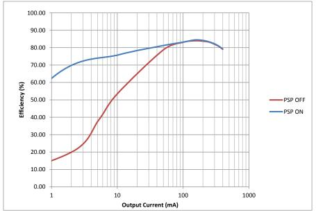
Figure 2. TPS65131 VPOS Efficiency
