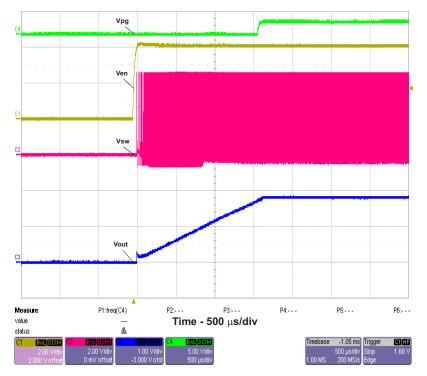
Figure 7. Power Up by Enable Pin Pulled High
