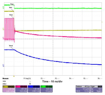
Figure 8. Power Down by Enable Pulled Low
