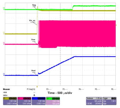
Figure 6. Power Up by Hot Plugging Vin
