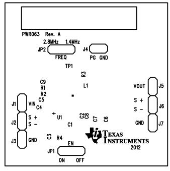
Figure 9. Assembly Layer
