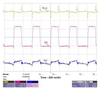
4.5V input, 1.8V output, 2.8MHz Switching; CH1: Input Ripple, CH2: Switching Node, CH3: Output Ripple
