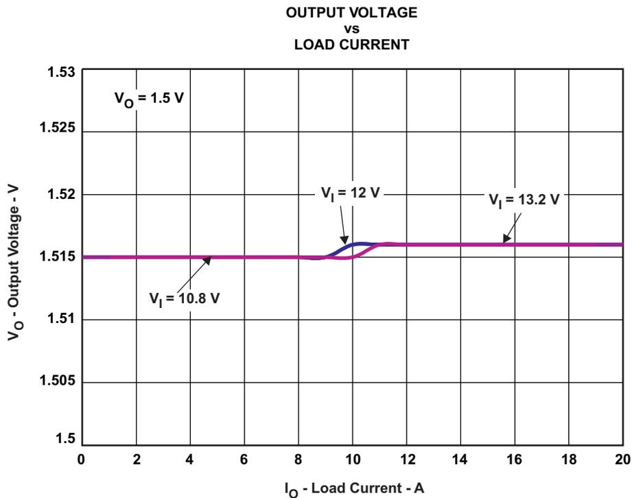
Figure 7. TPS40180EVM  $V_{OUT} = 1.5V$  Load Regulation
