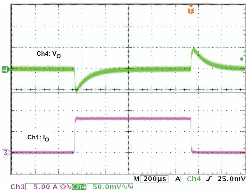
Figure 9. 0–8A Load Step, Ch1:  $I_{OUT}$  ; Ch4:  $V_{OUT}$
