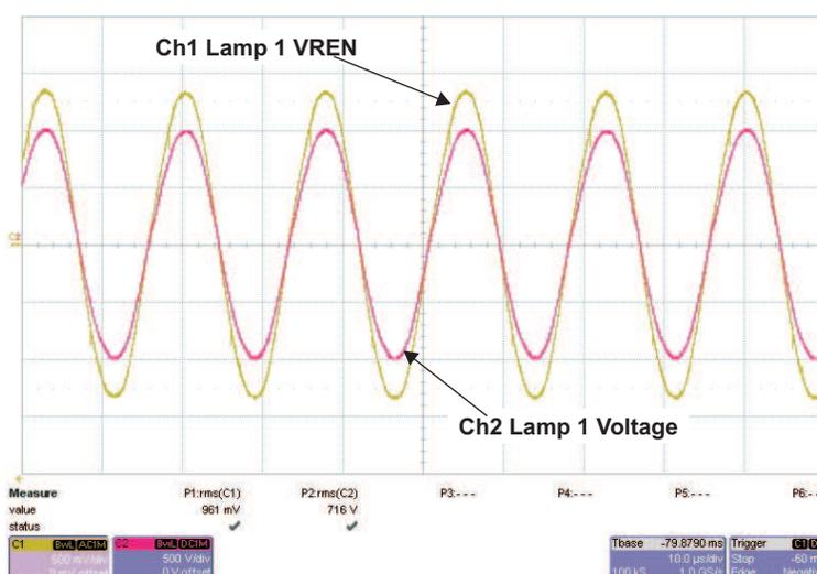
Figure 2. Lamp 1 VSEN Test Point Versus Lamp 1 Voltage
