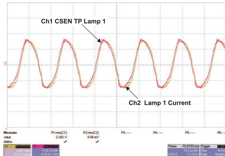
Figure 4. Lamp 1 CSEN Test Point and Lamp 1 Current
